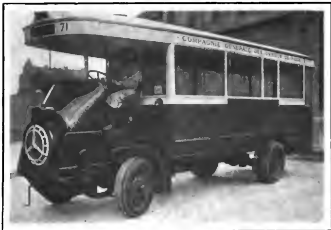
New Paris omnibuses have streamline effect with unbroken roof and scuttle dash
